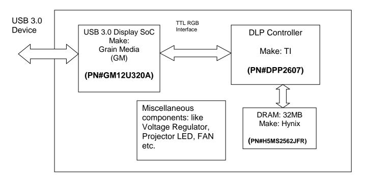
**Note:** Datasheets for Grain Media USB 3.0 controller and TI's DPP2607 are not available on the web. Block diagram is based on certain assumption made by author after looking at these products top level descriptions.
